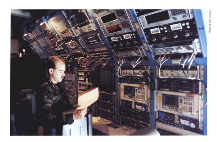
The mission crew sits on each side of a central aisle in what is, in effect, a broadcast studio located in the aircraft's cargo hold. All of the broadcast equipment is purchased off-theshelf, and thus the Guard can upgrade the equipment relatively easily as the technology improves. The aft two-thirds of the hold is filled with rows of transmitters, power supplies, and related equipment that go all the way to the paratroop door. Space is at a premium.
